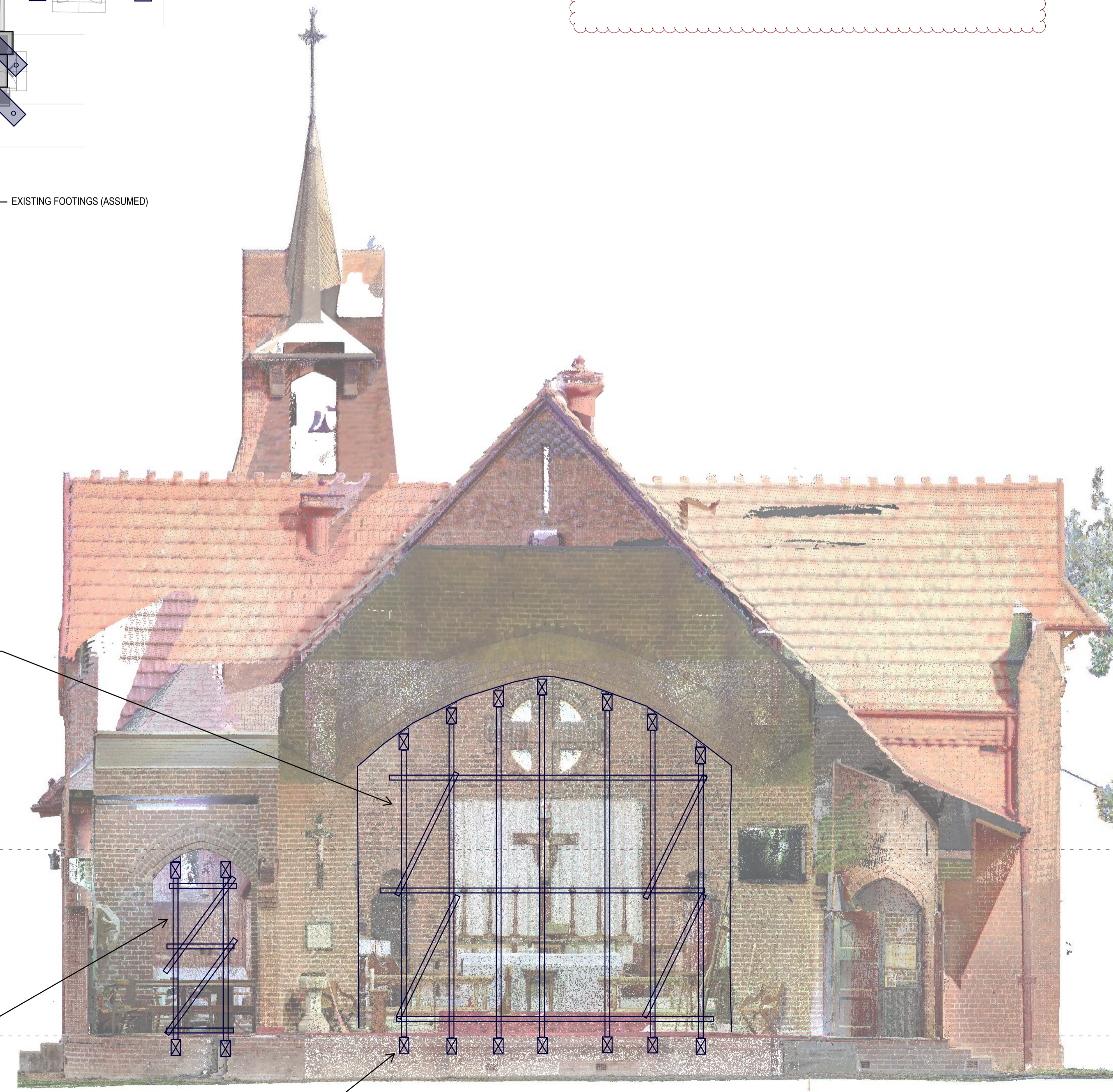
INDICATIVE MAIN ARCH PROPPING Scale 1:20
